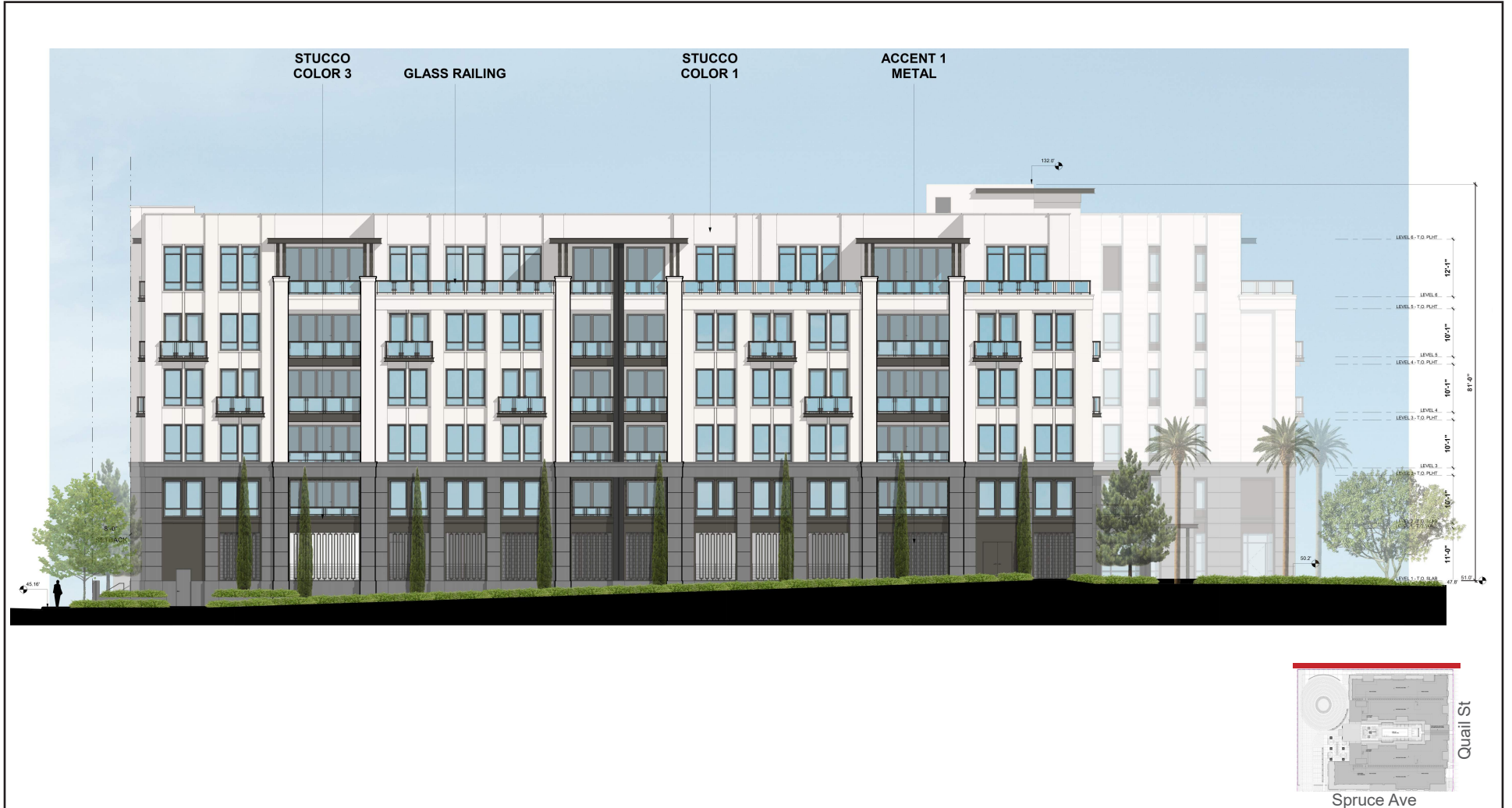
Figure 9c - Architectural Renderings (Northwest Elevation)
